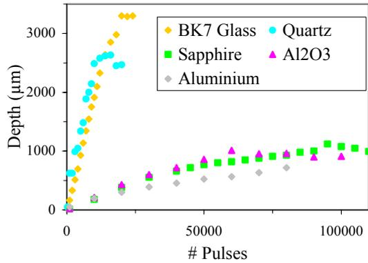
**Figure 7:** Maximum depth for different materials with a density of energy between 4.6 and 5.1 J/cm<sup>2</sup>.
