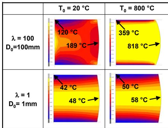
**Figure 9:** Workpiece size influence on forming temperature.
