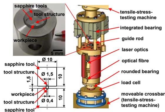
**Figure 11:** Exemplary tool-workpiece assembly and Experimental set-up.
