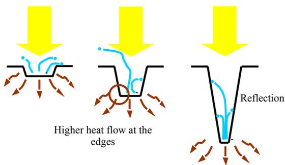
**Figure 5:** Modeling of deep drilling.
