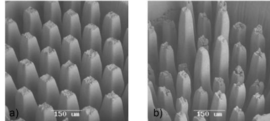
Figure 10a) Pyramidal structures in sapphire, with an aspect ratio of 5 (100  $\mu\text{m}$  to 500  $\mu\text{m}$ ) Figure 10b) and 10 (50  $\mu\text{m}$  to 500  $\mu\text{m}$ )
