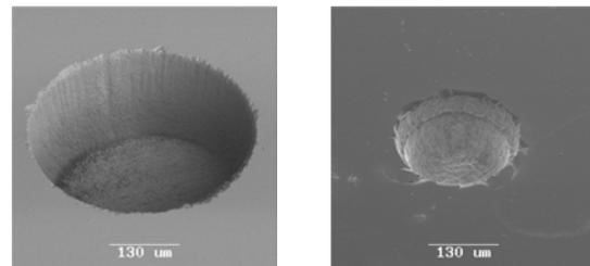
Figure 7: Increasing of micro-cracks in respect to a decreasing structure size
