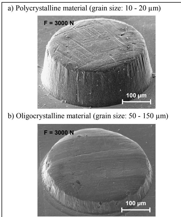
Figure 15: Semi-hot embossing (laser assisted forming with  $P_L = 6,7 \text{ W}$ ) of stainless steel
