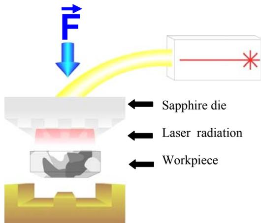
Figure 1: principle of the laser assisted microforming process with laser structured sapphire dies
