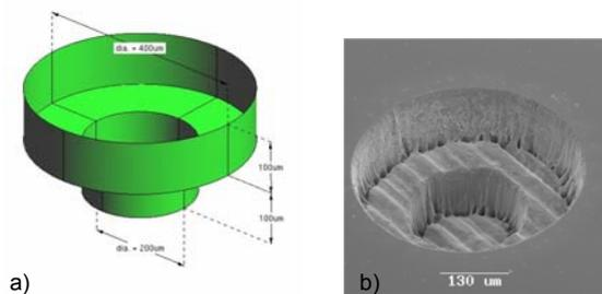
Figure 3: a) drawing of the required structure
