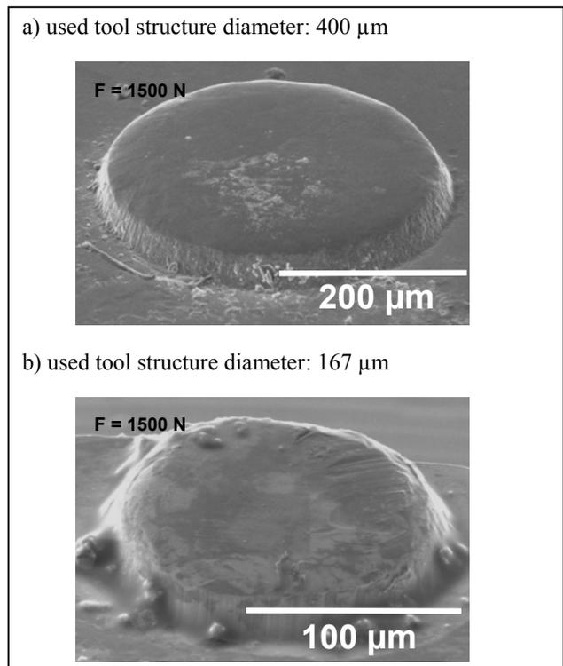
Figure 16: Formfilling of scaled tool structures with polycrystalline material (grain size: 10 – 20  $\mu\text{m}$ )
