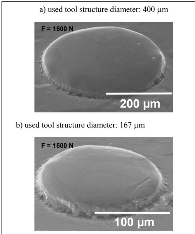
Figure 17: Formfilling of scaled tool structures with oligocrystalline material (grain size: 50 - 150 μm)
