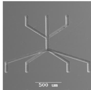
Figure 18: Microfluidic system in sapphire
