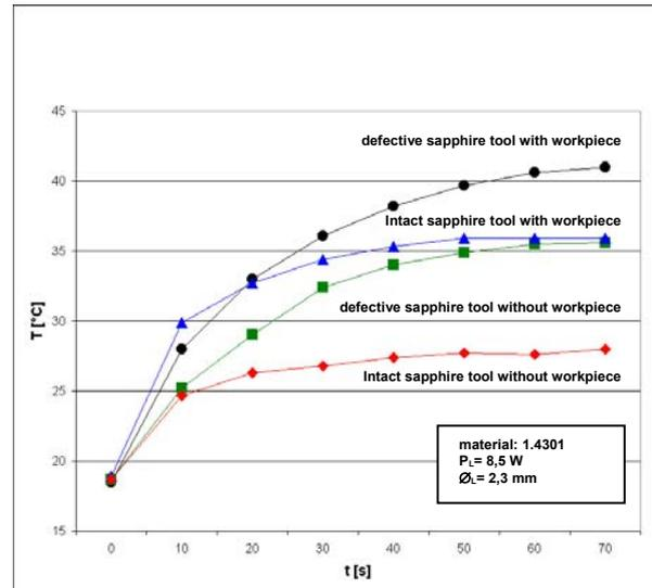
Figure 13: sapphire tool heating depending on the condition of the sapphire tool with and without workpiece contact
