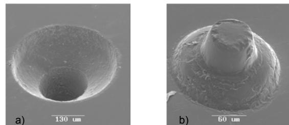
Figure 4: a) twin-cylinder, structured with excimer laser  $\lambda = 193 \text{ nm}$ , imaging procedure,
