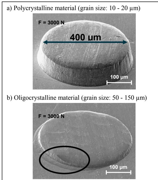
Figure 14: cold embossing of stainless steel
