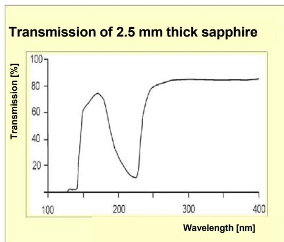
Figure 2: Transmission curve of sapphire
