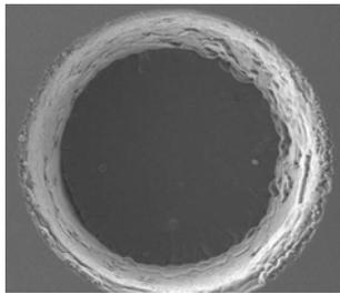
Figure 8: 300 $\mu\text{m}$  deep drilling in a 350  $\mu\text{m}$  thick sample
