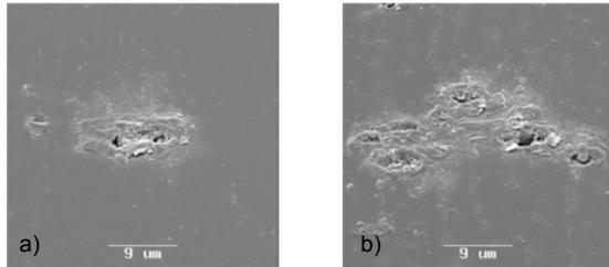
Figure 9: Damaging of the sapphire sample backside induced by interference of the non-absorbed radiation at a residual thickness of 80  $\mu\text{m}$  (9a) and 50  $\mu\text{m}$  (9b).
