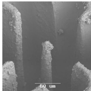
Figure 11: Structure generated with Excimer radiation (193 nm), diameter of the tip on the top: 20  $\mu\text{m}$
