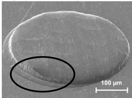
**Figure 9:** Cold embossing of stainless steel
