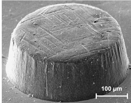
b) Oligocrystalline Material (grain size: 50 - 150  $\mu\text{m}$ )
