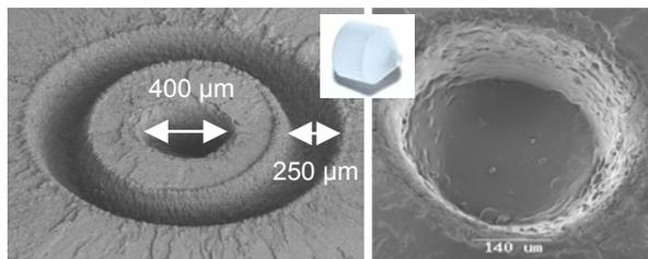
**Figure 4:** Sapphire tool for embossing experiments
