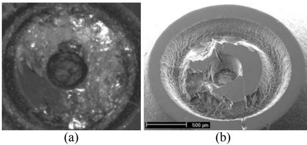
**Figure 7:** Sapphire tool fractured during the embossing experiments ( $F = 5000 \text{ N}$ ,  $P_L = 20 \text{ W}$ )
