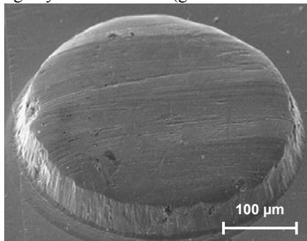
**Figure 10:** Semi-hot embossing (laser-assisted forming with  $P_L = 20 \text{ W}$ ) of stainless steel
