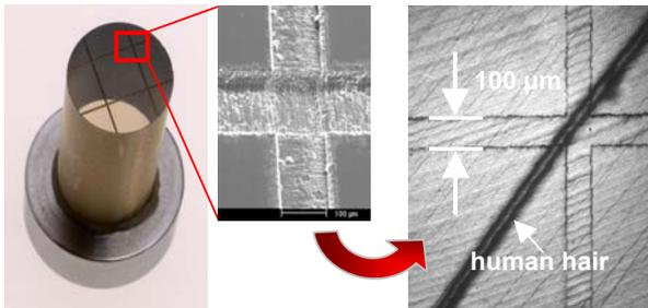
**Figure 3:** Prototype of a sapphire tool for embossing and imprint in aluminum in comparison with a human hair
