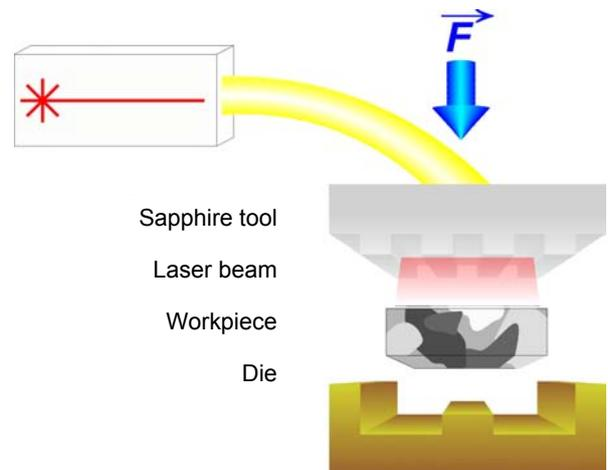
Figure 1: Principle of laser-assisted microforming
