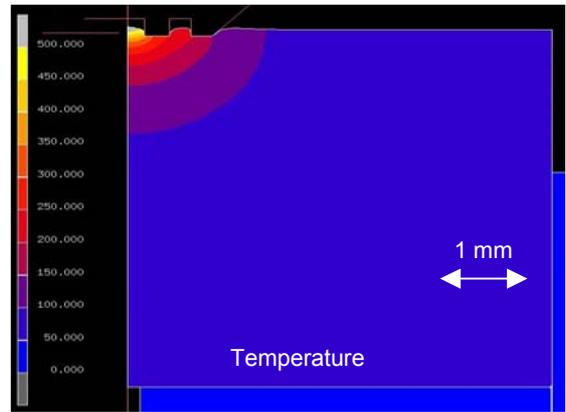
**Figure 5:** Results of FE simulations of the embossing experiments ( $F = 5000\ \text{N}$ ,  $P_L = 20\ \text{W}$ )
