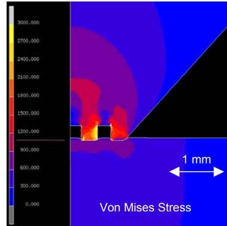
**Figure 8:** Results of FE simulations of the embossing experiments ( $F = 5000 \text{ N}$ ,  $P_L = 20 \text{ W}$ )
