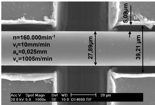
**Figure 13:** Groove in brass CuZn37 with inserted optical fiber produced with a diamond micro side milling cutter
