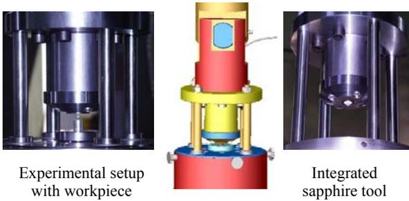
**Figure 2:** Prototype of a setup for laser-assisted microforming
