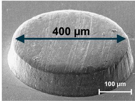
b) Oligocrystalline Material (grain size: 50 - 150  $\mu\text{m}$ )
