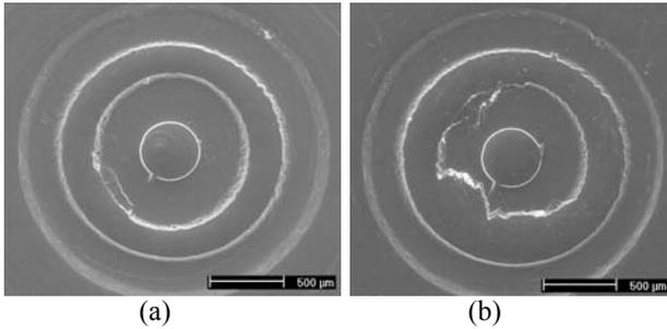
**Figure 6:** Results of the embossing experiments: imprints in stainless steel 1.4301 ( $F = 5000 \text{ N}$ ,  $P_L = 20 \text{ W}$ )
