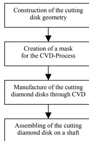
**Figure 11:** Development phases of the diamond micro side milling cutter
