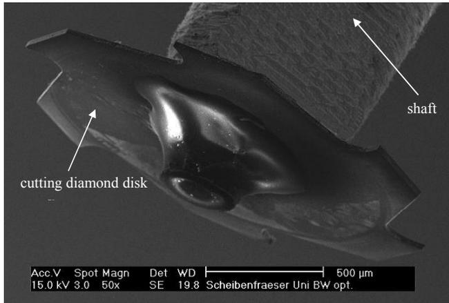
**Figure 12:** Installed diamond micro side milling cutter
