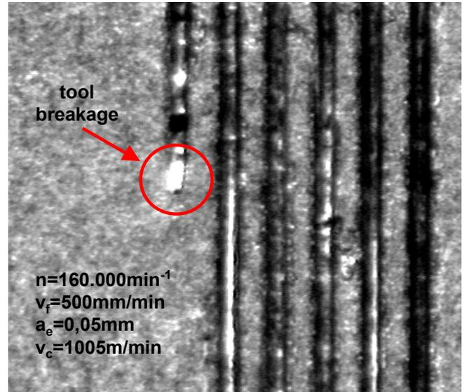
**Figure 14:** Grooves in stainless steel (1.4301) produced with a diamond micro side milling cutter
