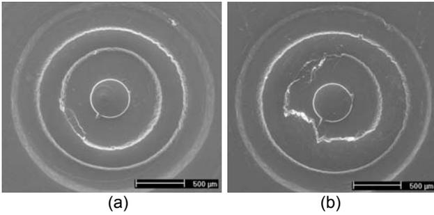
Figure 6: Results of the embossing experiments: imprints in stainless steel 1.4301.
