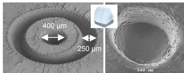
Figure 4: Sapphire tool for embossing experiments.
