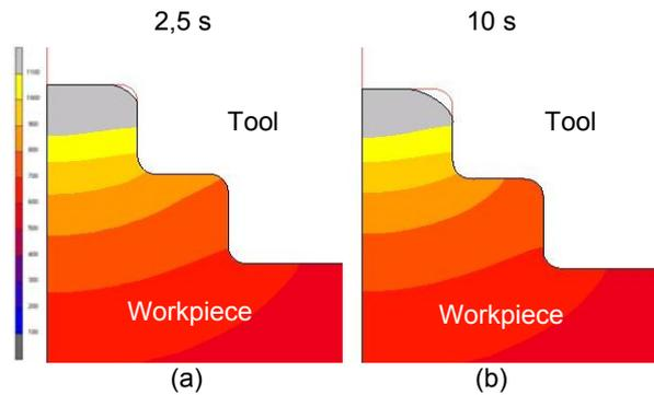
Figure 10: Form filling after fast (left) and slow (right) heating.
