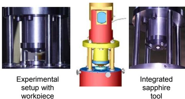
Figure 2: Prototype of a setup for laser-assisted microforming.
