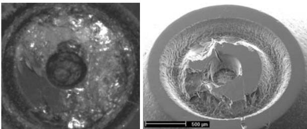
Figure 7: Sapphire tool fractured during the embossing experiments.
