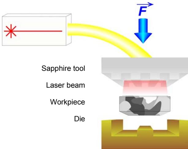
Figure 1: Principle of laser-assisted microforming.
