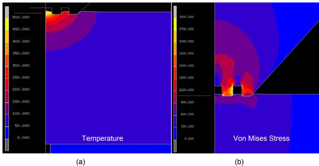
Figure 5: Results of FE simulations of the embossing experiments.
