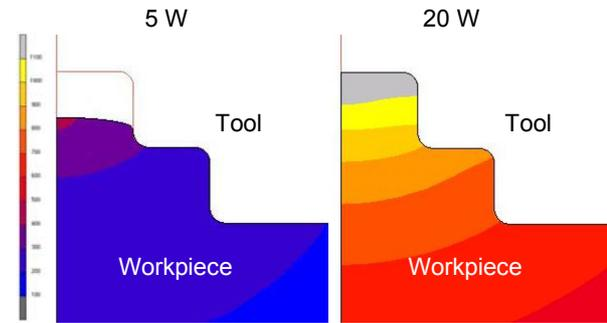
Figure 9: Form filling of the workpiece at different laser power.
