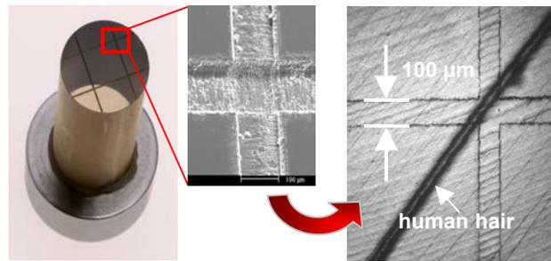
Figure 3: Prototype of a sapphire tool for embossing and imprint in aluminium in comparison with a human hair.
