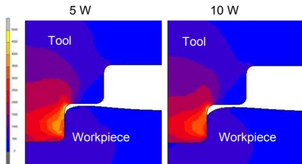
Figure 11: Tool stress at different laser power.
