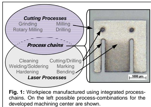
Fig. 1: Workpiece manufactured using integrated process-chains. On the left possible process-combinations for the developed machining center are shown.
