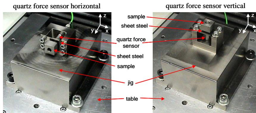
Fig. 2 Improved Prototypes of a force measurement system of the LaFT
