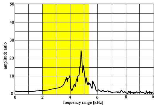
Fig. 1 Natural frequencies of the "MiniDyn Type 9256A2" in the x-axis [1] and excitation frequencies based on micro machining operations
