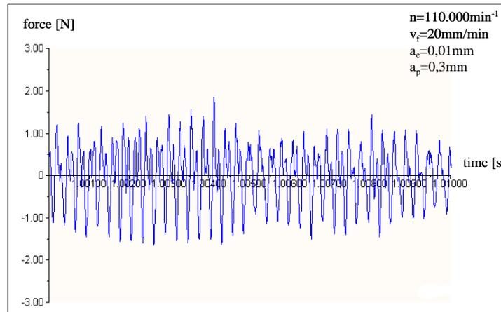
**Fig. 4** Force progression in the y-axis for 10ms during milling
