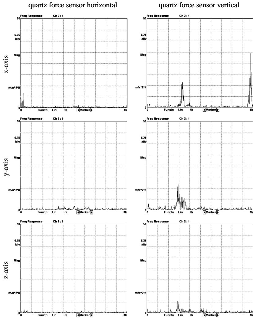
Fig. 3 Transfer functions in the x-, y- and z-axis
