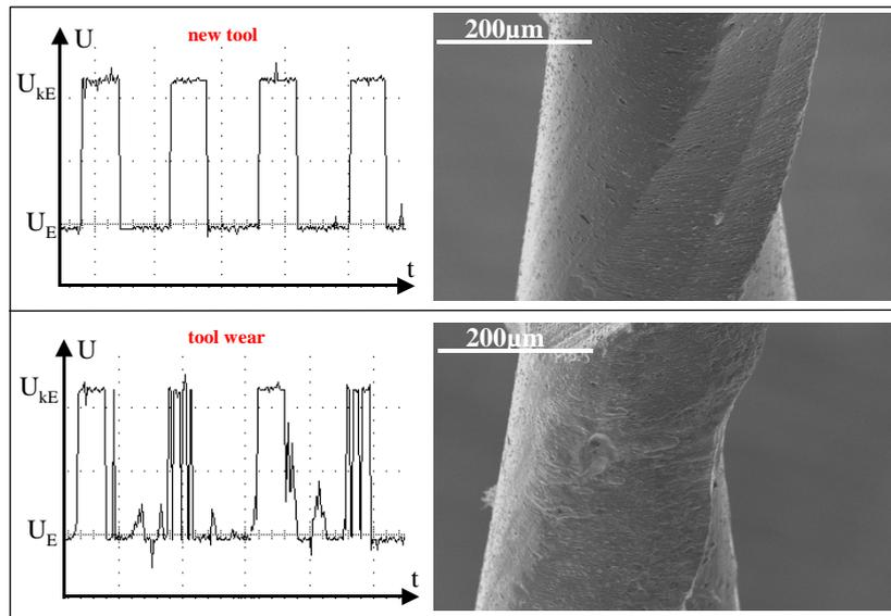
Figure 4: Inprocess detection of tool wear with Transition Resistance Sensor
