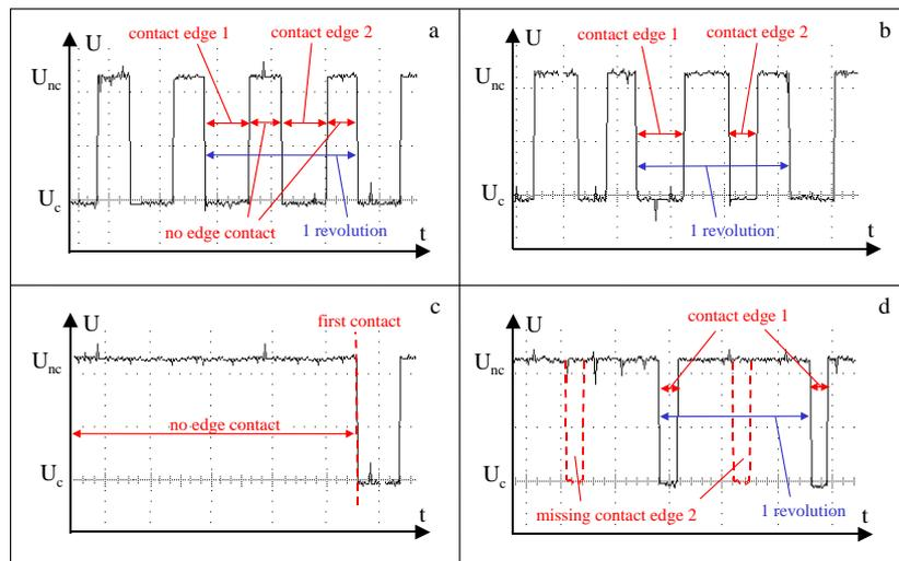
Figure 3: Possible monitoring options of the new Transition Resistance Sensor
