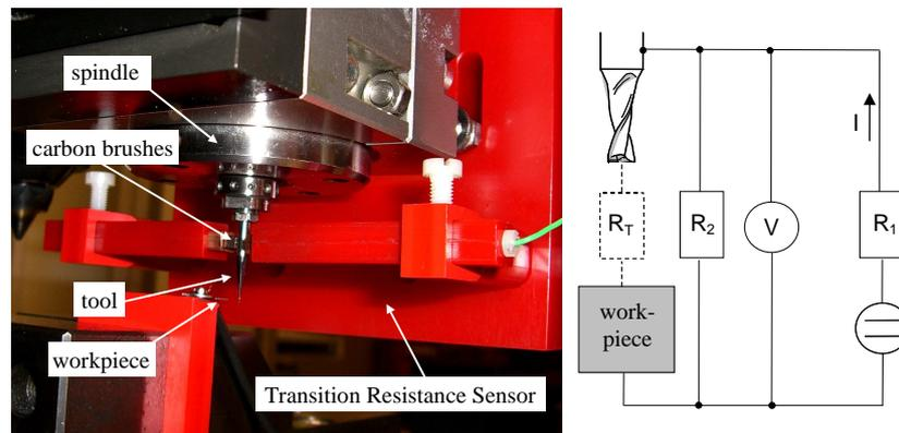
Figure 1: Transition Resistance Sensor and its functional principle
